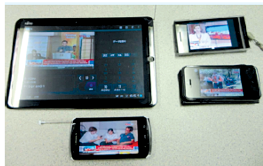
Figure 2-5-3: Mobile Terminals That Receive ISDB-T Narrow Broadcast and IPTV streaming Over Wi-Fi in the Testbed Site.
